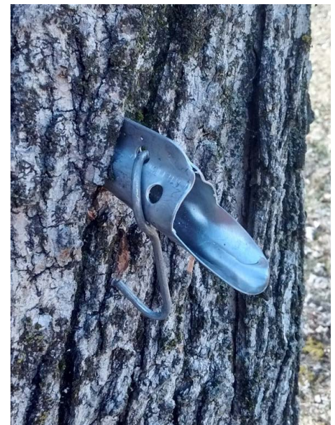
Many different kind of spiles are available. This is the most common spile, designed to hang a bucket on to collect the sap.
