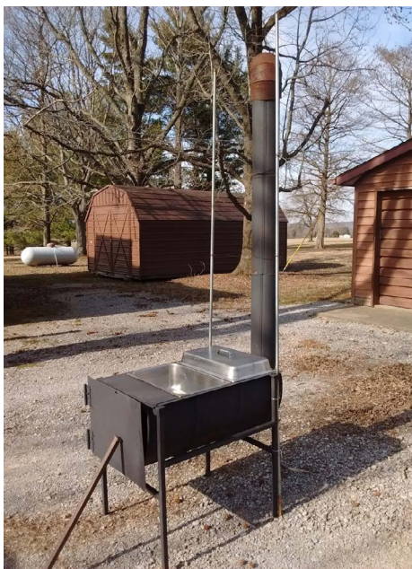
A simple homemade wood-fired boiler. Commercial evaporators are also available for purchase.
